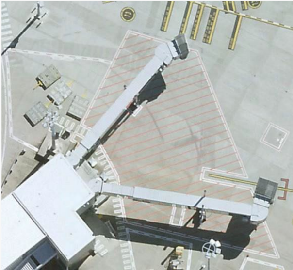
Figure 23 Red Hatching Lines – Safety Areas
