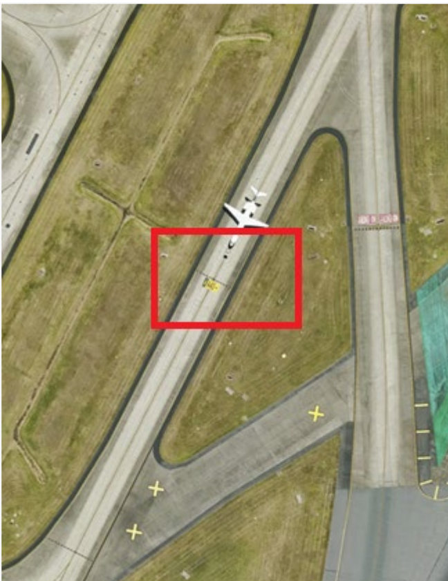
Figure 60 Enhanced Intermediate Holding Positions at Rapid Exit Taxiways (RETs) – TWY A4S and TWY A6
