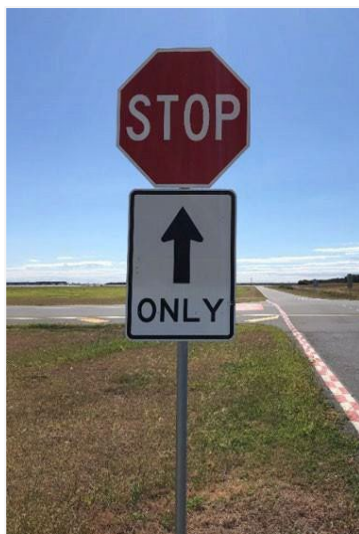
Figure 18 Taxiway Crossing Stop Sign Example
