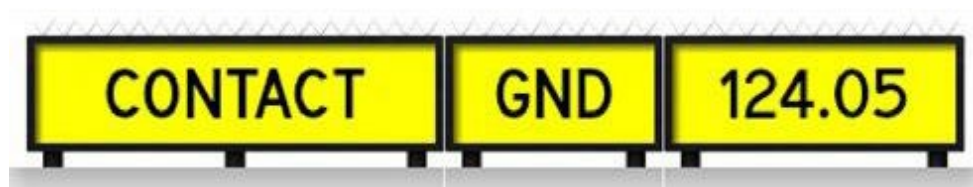
Figure 55 Example of Ground Frequency Change MAG Sign
