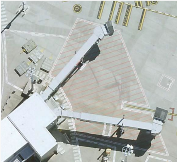
Figure 23 Red Hatching Lines – Safety Areas
