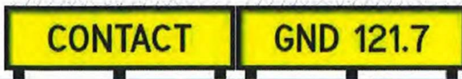
Figure 58 Example of Ground Frequency Change MAG Sign
