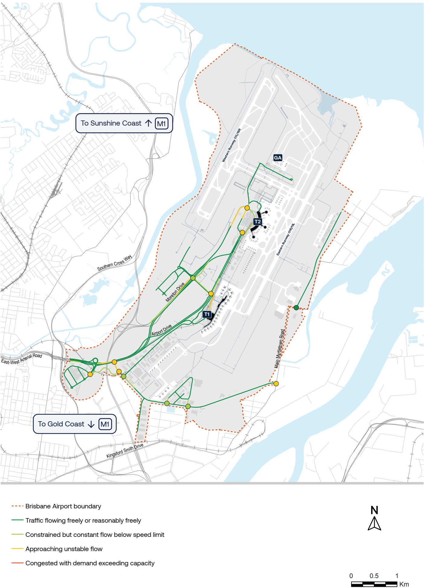
FIGURE 14.9: ON-AIRPORT CURRENT PEAK HOUR TRAFFIC
