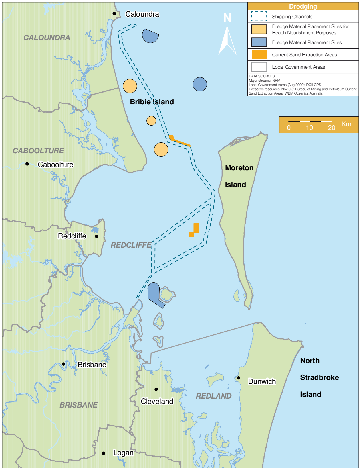
Figure 1.2: Location of Existing Commercial Extraction Permit Areas, Dredge Placement Sites and Maintained Shipping Channels in Moreton Bay.
