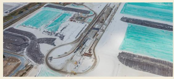
2. 700 piles anchor and support the structure. These are mostly in lots of 3 x 12m segments, to an average depth of 30m below ground.
