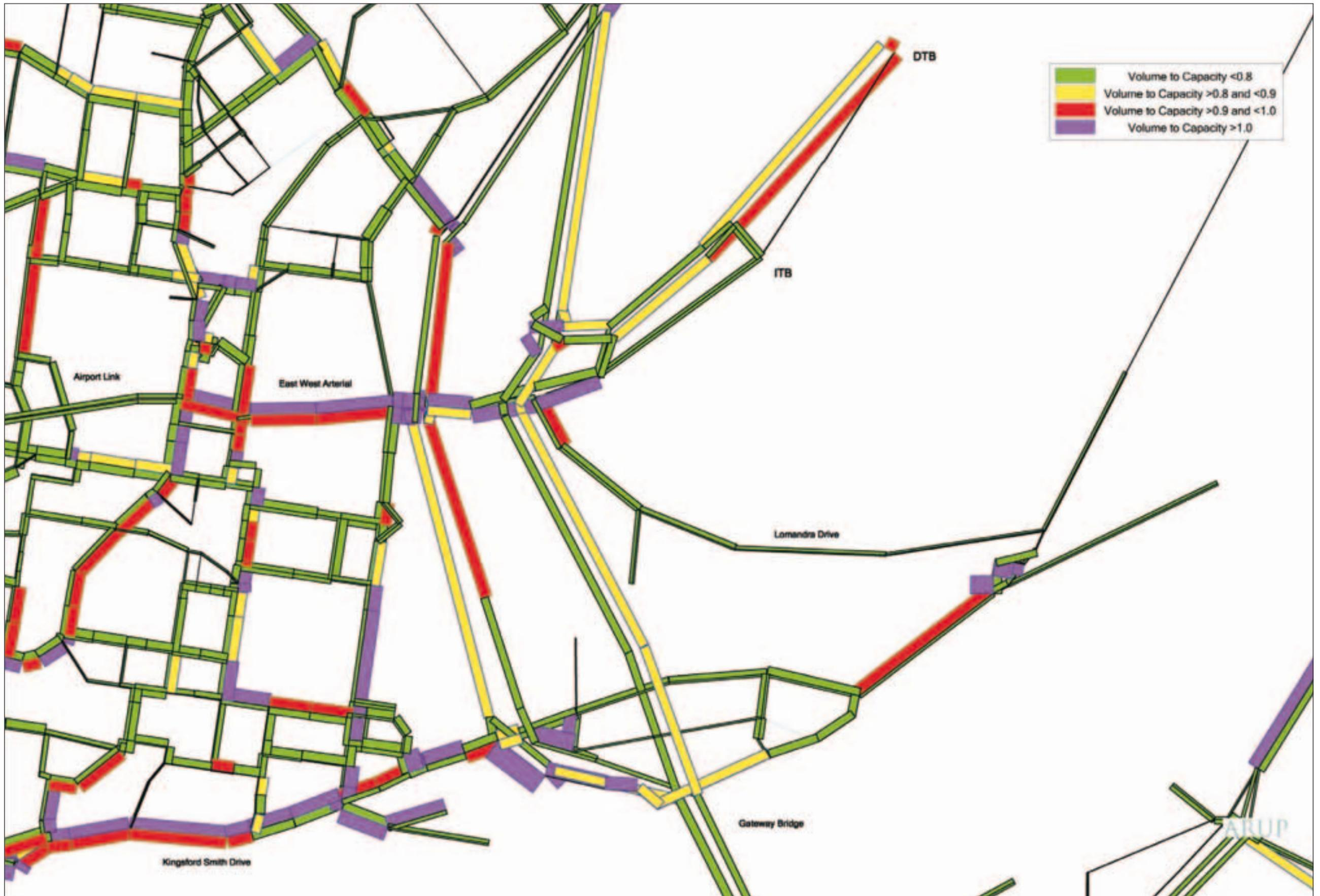
Figure 10.9b: Volume to Capacity Ratio 2035 NPR PM Peak (4pm-6pm)
