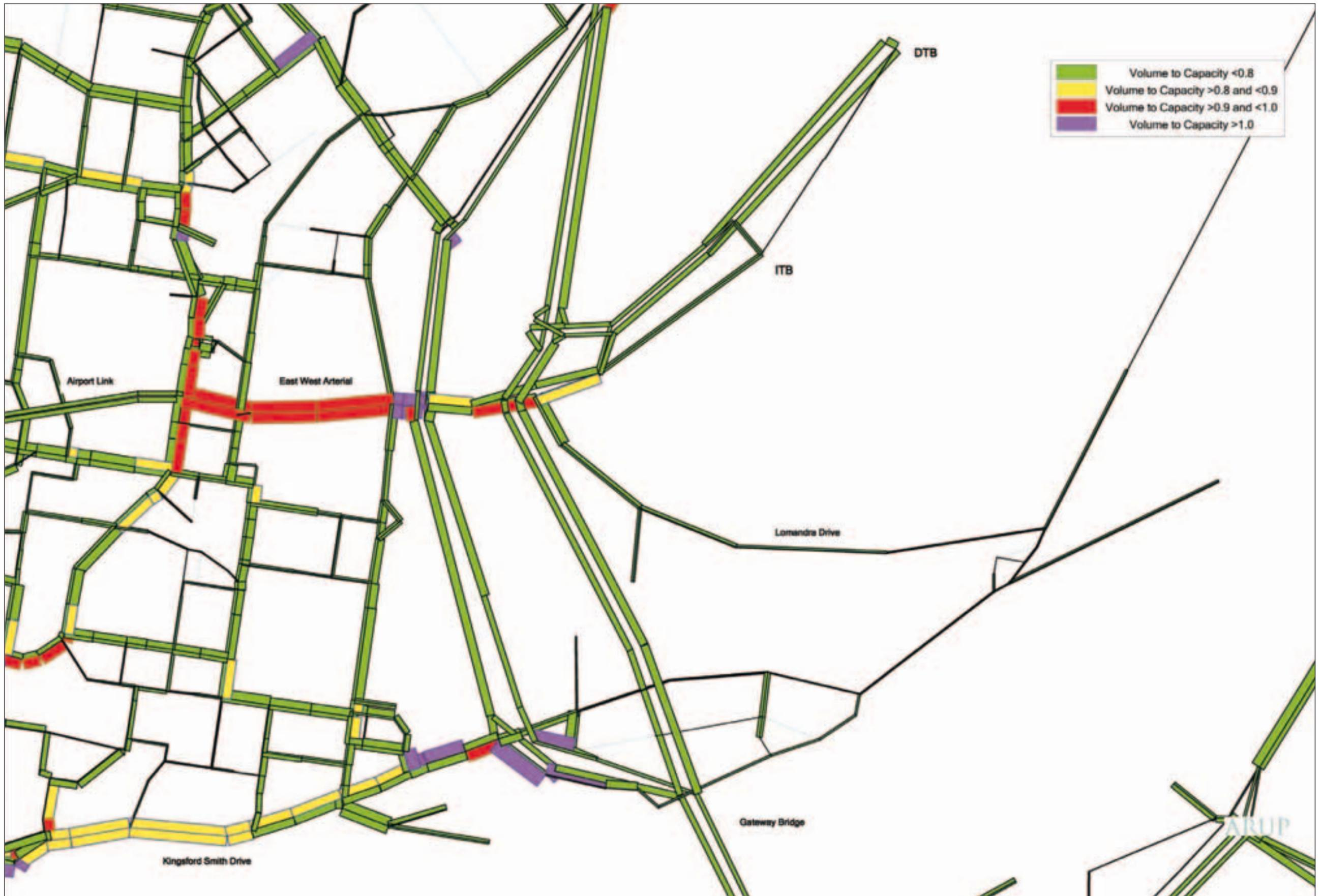
Figure 10.7c: Volume to Capacity Ratio 2015 Base PM Peak (4pm-6pm)
