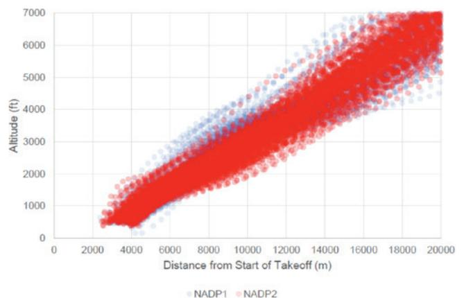
While the trial was conducted off the existing runway, the following diagram transfers the trial aircraft across to the new runway to show aircraft altitudes at distances from the point of take-off over residential areas. It also shows the two noise abatement departure procedures and the area of potential improvement the trial investigated.
