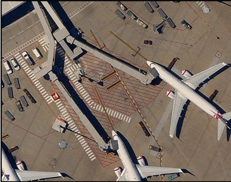
Figure 21 Red Hatching Lines - Safety Areas
