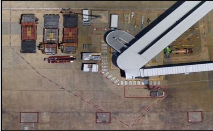
Figure 18 Single Broken Red Line - Staging / Clearance
