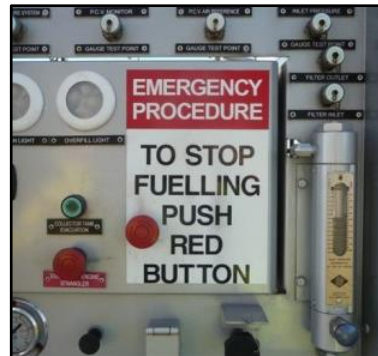
Figure 10 Emergency stop on vehicle
