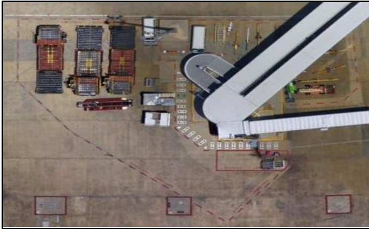
Figure 21 Single Broken Red Line - Staging / Clearance
