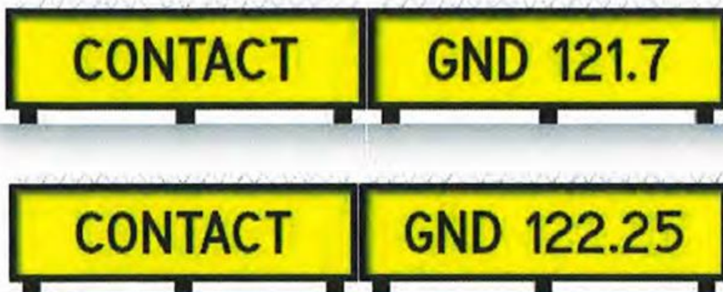
Figure 52 – Ground Frequency MAG Signs
