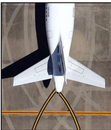
Figure 48 Parking Clearance Line
