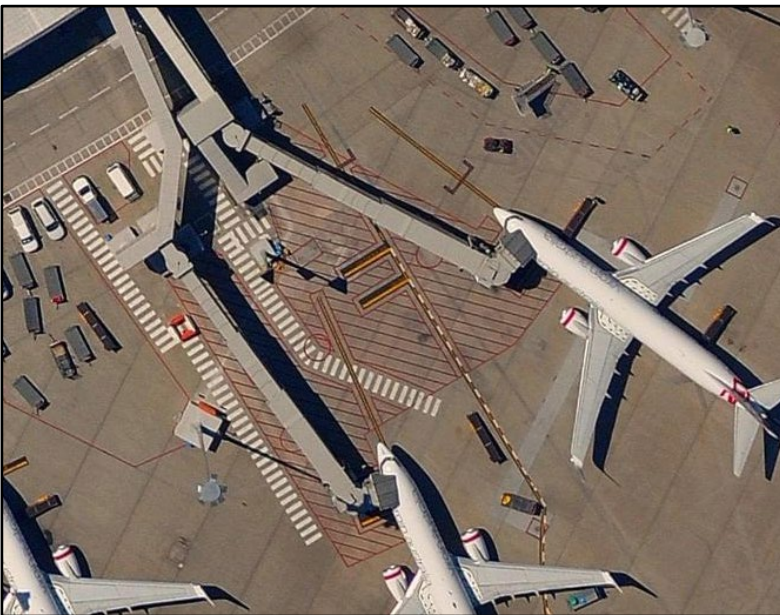
Figure 22 Red Hatching Lines - Safety Areas
