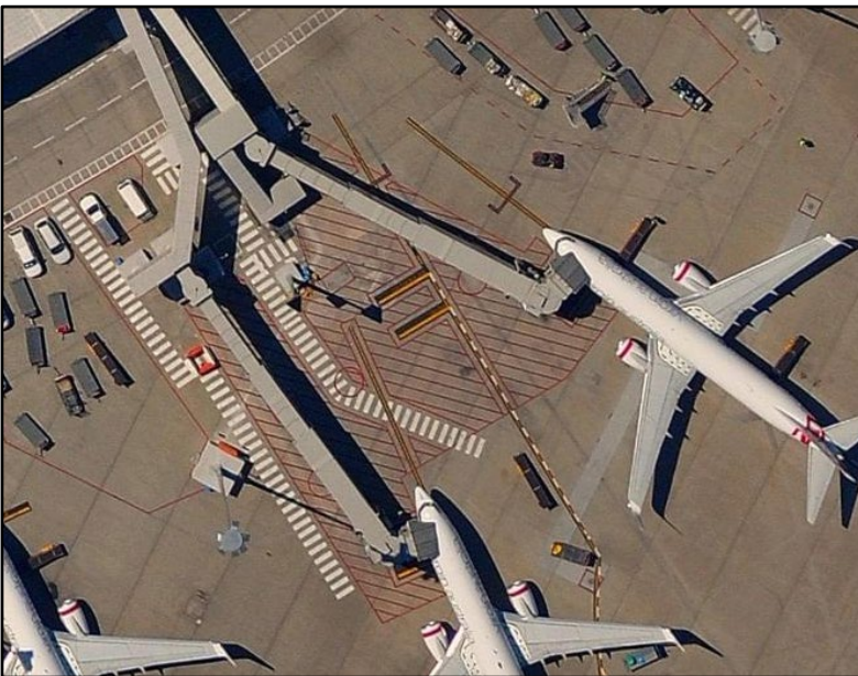
Figure 22 Red Hatching Lines - Safety Areas
