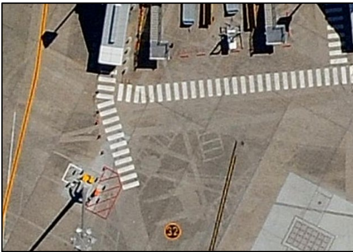
Figure 7 Pedestrian walkway and hatched eye wash station
